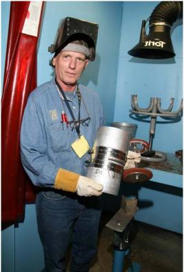
This course emphasized "how to teach" Gas Tungsten Arc Welding in order to increase the quality and quantity of UA instructors in our local welding programs. The course consisted of welding pipe in the 2G, 5G and 6G positions.
